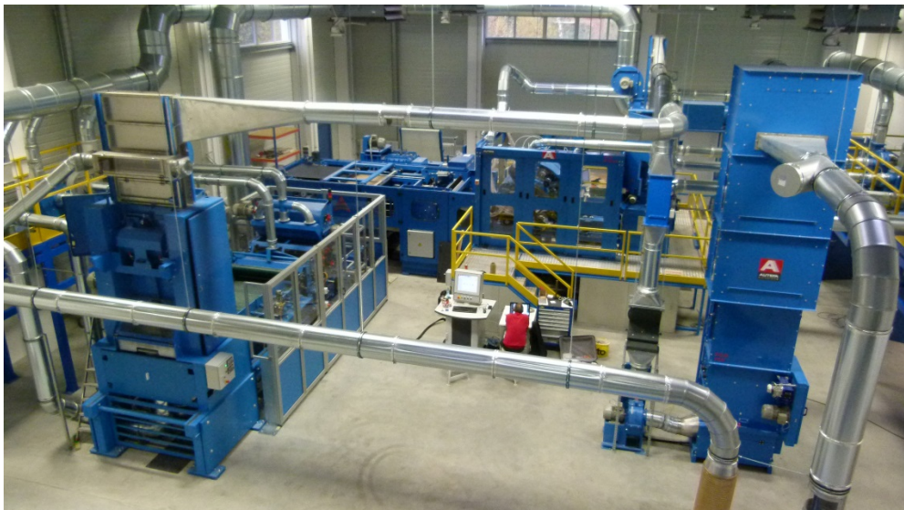
Nonwoven line during start-up phase (left: Airlay process, right: carding process (source: STFI ))
