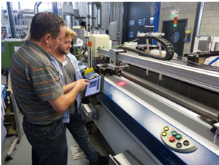
Process control using Assistance Systems on Smart Mobile Devices (source: ITA)
