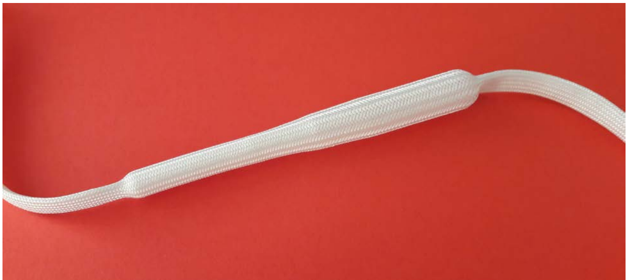
Uncoated artificial ligament structure comprised of a liquid silicone rubber core and overbraided with PET
