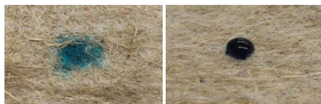
Figure 2: Nonwoven made from flax fibers, untreated (left) and treated with a hydrophobization agent from natural resources (right)
