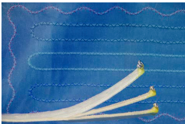
Adaptive FRPCs with structurally integrated actuators (© ITM/TU Dresden)
