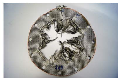
Pressure shock test (3 layers coated Vectran®; burst pressure: 70,1 bar)
