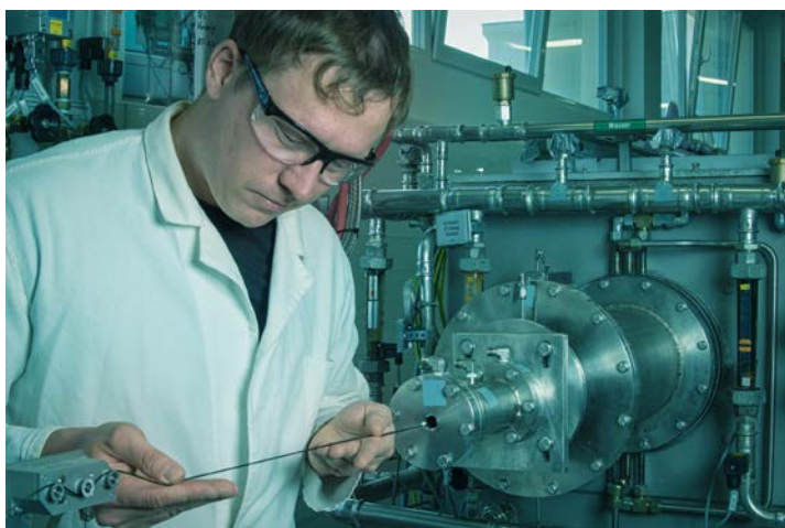
Dr. Martin Kirsten, Research Group Head at the ITM, and the institute's Stabilization and Carbonization Unit for the production of carbon fibers (©: ITM/TU Dresden)
