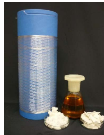
Figure 1: IL-spun precursor fiber based on cellulose
