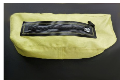
Pressure shock test (3 layers coated Vectran®; burst pressure: 70,1 bar)
