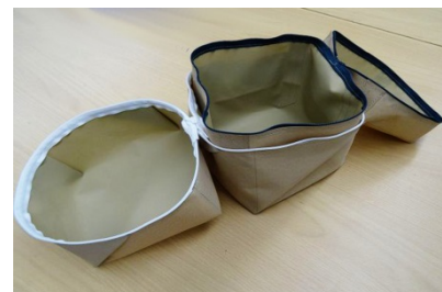
Designs of a blast resistant textile based bags (reference: ITM, Dresden)
