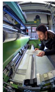
Multiaxial warp knitting machine with warp yarn manipulation module for the production of biomimetic multifunctional textile reinforcements Source: TU Chemnitz/MERGE, Photo: Hendrik Schmidt
