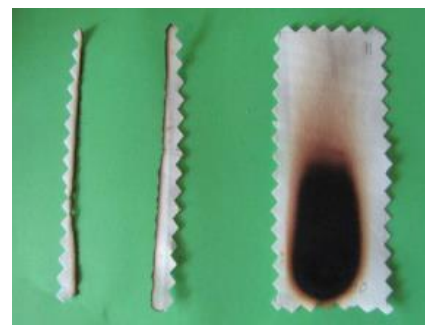
Fig. 2: Flammability test on cotton fabric (left: blank, right: polyphosphazene-modified)
